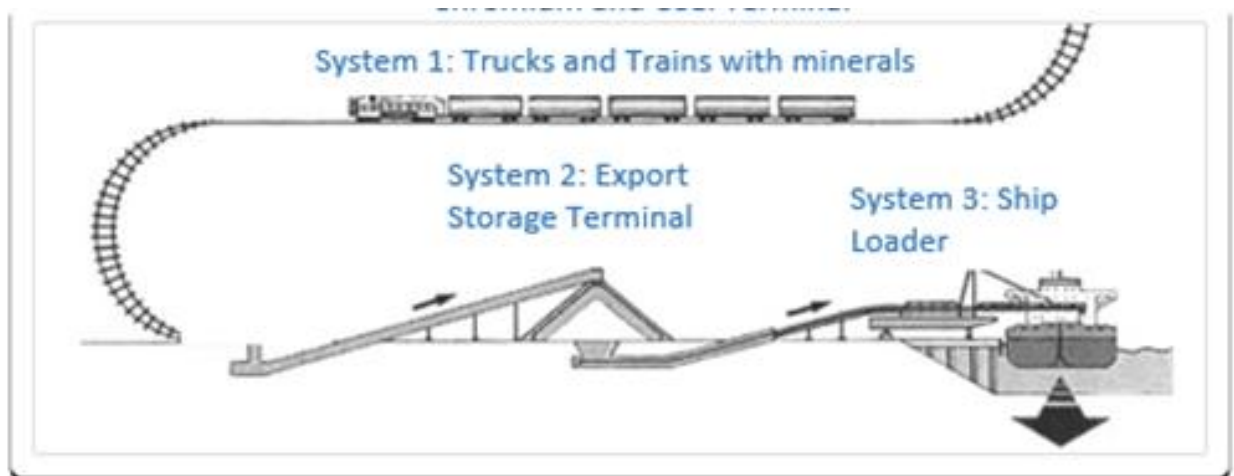
Figure 6: Chromium and Coal main systems terminal
