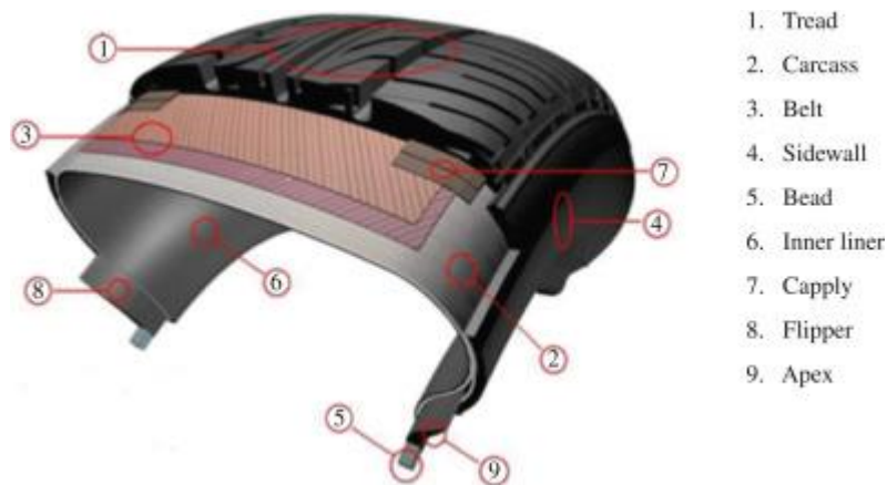
Figure 7: Basic structure of tire
